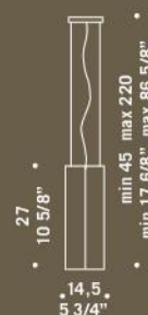
CARRÈ S1P 1x70W E27 HSGSA/C alogeno chiara clear halogen 1x26W E27 FBT fluorescente fluorescent
