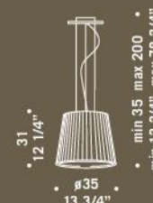
LUMÈ S1 1x70W E27 HSGSG/C alogeno Globolux chiara clear halogen Globolux 1x70W E27 HSGSA/C alogeno chiara clear halogen
